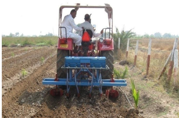
Testing of tractor drawn BBF planter
