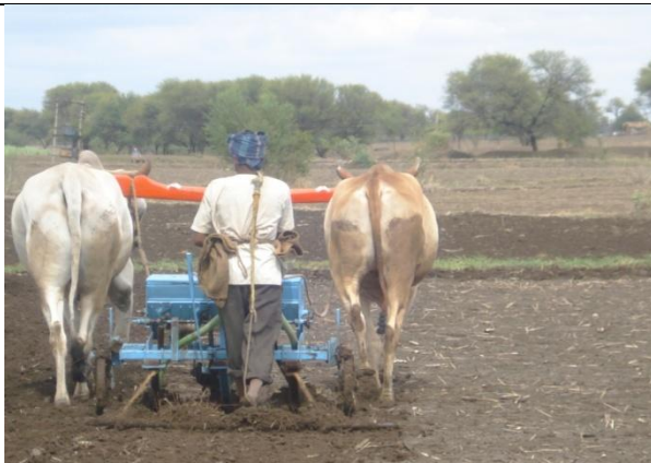
Frontline demonstration of refined CRIDA bullock drawn planter
